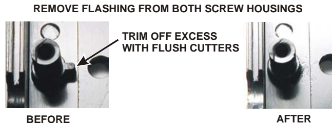
Figure 17. Removing Excess Plastic From Enclosure Top Cover.
